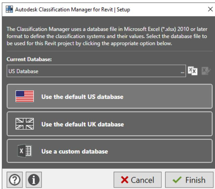
The user can return to this screen to change the selection at any point during the project lifecycle, if necessary. The name of the database chosen is saved in the extensible storage of the RVT file. Instructions on creating a custom classification database can be found in the Excel file, "Classification Manager Database Custom.xlsx" located in the Classification Manager installation folder.
