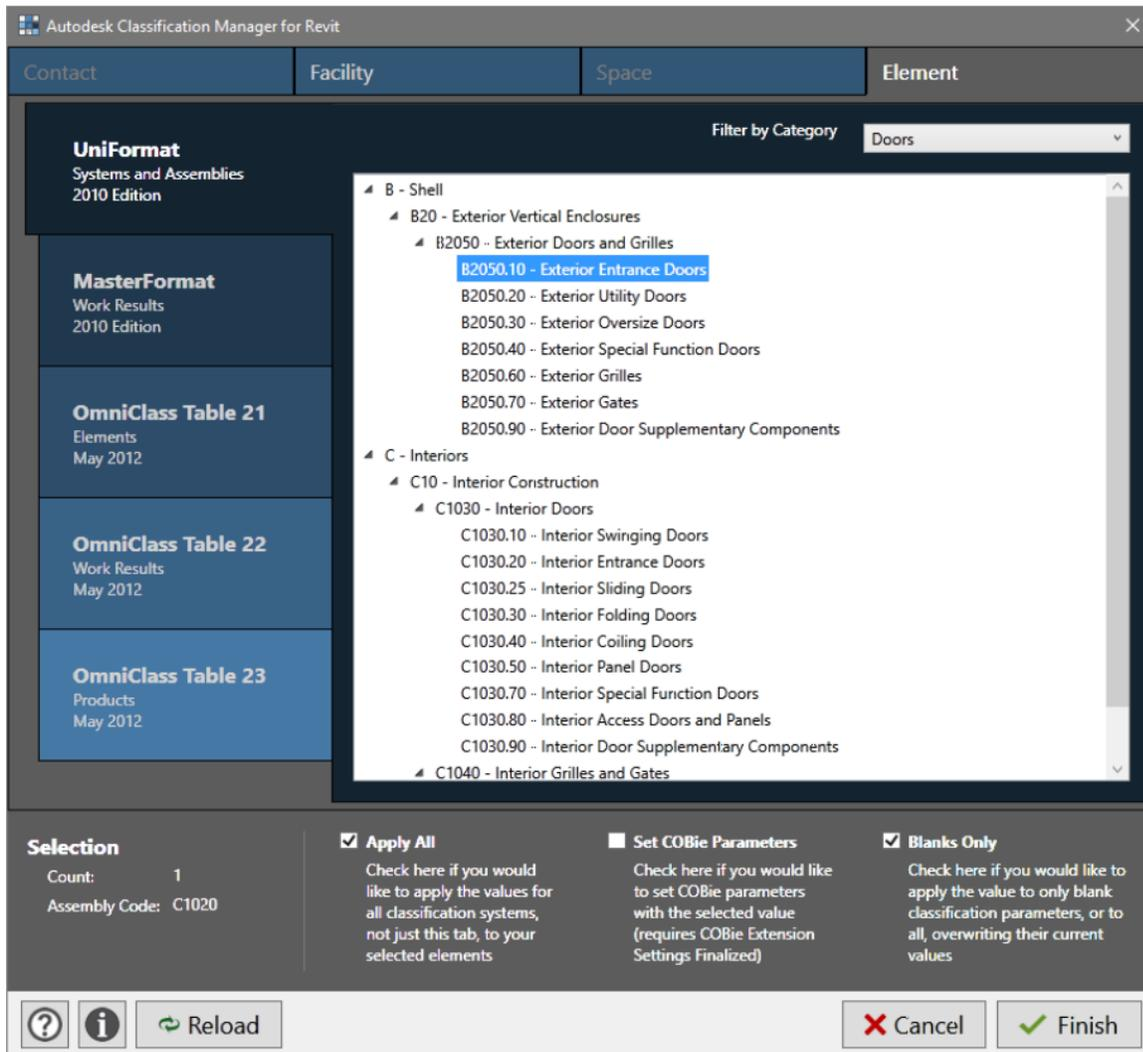
The user can simply navigate through the tree in the right-hand window, select the wanted classification, and click the “Finish” button. One can easily toggle between classification systems on the left if the database supports multiple systems. If the chosen database has been set up to support cross classifying, the "Apply All" checkbox
