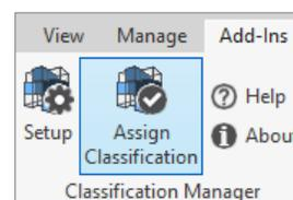
Depending on what type of element is selected, the appropriate tab and filter will be applied to limit the classifications shown to those related to the selection.
